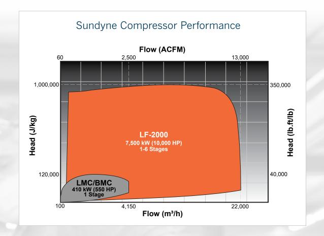
Please consult Sundyne to confirm compressor performance, as gas composition has a significant influence on thermodynamic properties and thus the developed head and efficiency.
