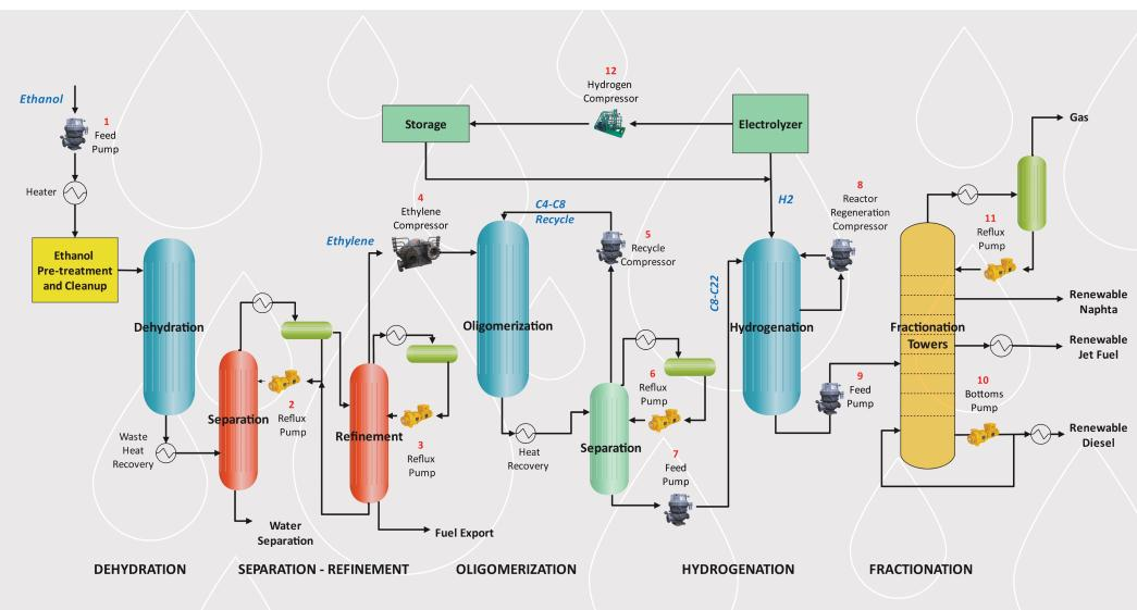
Note, any source of hydrogen can be used in alcohol-to-jet SAF production. Here, we show green hydrogen produced via electrolysis
