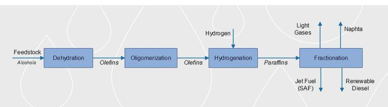
Typically, the Alcohol-to-Jet fuel conversion process includes the following steps:
