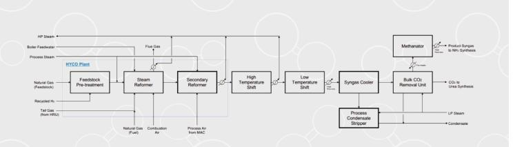
Generic Block Flow Diagram of the syngas generation IEAGHG, "Techno-Economic Evaluation of Hyco Plant Integrated to Ammonia/Urea or Methanol Production with CCS", 2017/03, February, 2017
