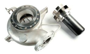
Constructed from a composite material of poly-ether-ether-ketone (PEEK) and carbon fibre, the ZeroLoss Containment Shell facilitates better handling of volatile and heat sensitive fluids and helps improve reliability.
