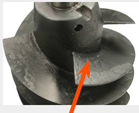
Advanced metal corrosion due to cavitation; under the wrong conditions, cavitation reduces the equipment lifetime dramatically.
