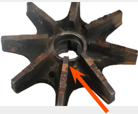
Advanced metal corrosion due to cavitation; under the wrong conditions, cavitation reduces the equipment lifetime dramatically.
