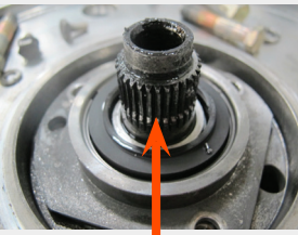
Up thrust failure from non-OEM "re-manufactured" high speed bearing.
