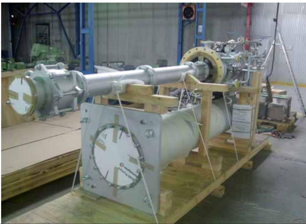
➤ **Sealing** on the shaft can be done either by a stuffing box or mechanical seal, as required.
