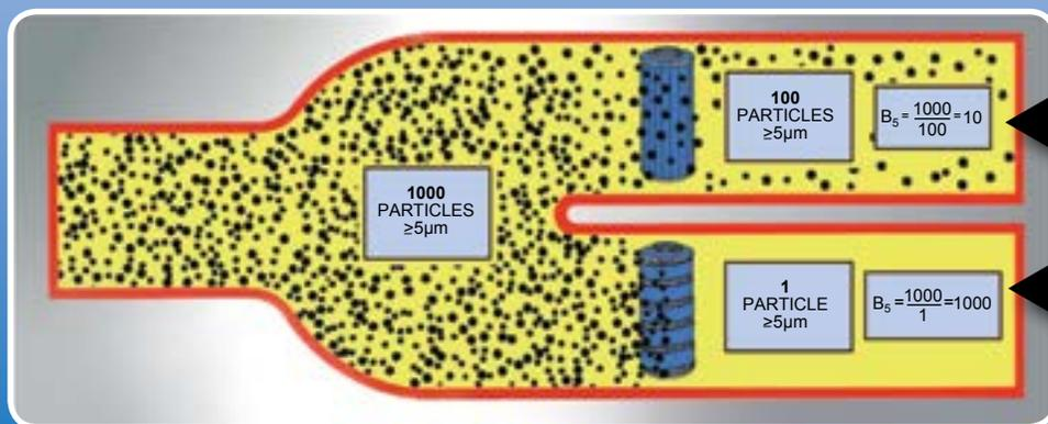
**Typical 5µm Nominal Non-OEM Filters**
