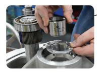
Bearing Plate The redesigned bearing plate improves oil path flow and accommodates the new heavy duty internal components. Anti-Friction Bearings The upgraded antifriction bearing set increases efficiency and shaft longevity.
