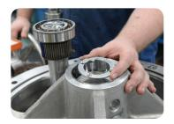
Lube Oil Pump & Anti-Rotation Plate An improved internal lube oil pump locks securely in place, using our newly designed anti-rotation plate, which can tolerate much higher radial shaft loads.
