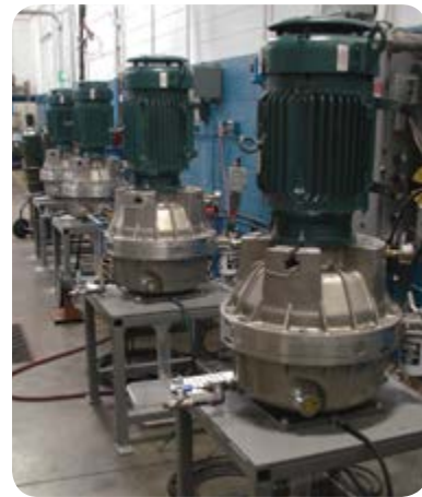
Seal Validation Program With Multiple Test Rigs
