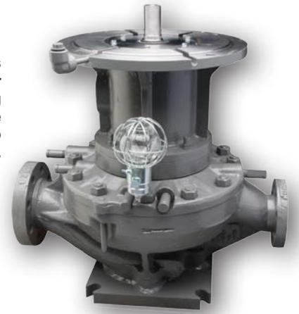
The Sundyne LMV-801 API 610, is a direct drive vertical inline, single stage, overhung impeller centrifugal pump in a standard OH5 configuration. OH3 when used with the bearing frame option. This model delivers:
