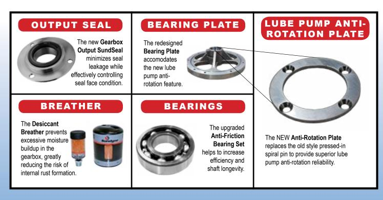
Comprised of an improved lube pump drive mechanism, the new gearbox output SundSEAL, our desiccant breather and an upgraded anti-friction bearing set, the Sundyne Gearbox Reliability Upgrade Kit is the easiest way to improve the performance of your existing Sundyne gearbox without the need for a replacement.
