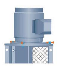
Transverse alignment positioning **jackscrews** for electric motor
