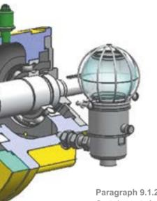
**Paragraph 9.1.2.1.1** Containment shell – constructed in accordance with ASME VIII international standards.
