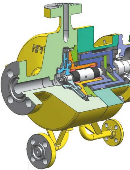
KEY **Pump Casing** Magnetic Drive Impeller **Bush Holder Bump Ring** Silicon Carbide Bushes Silicon Carbide Shaft Sleeves **Power Frame** and Thrust Washers
