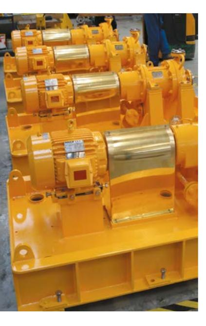
The HPGSP range comprises pumps based on the Sundyne HMD Kontro GS drive, built to API 685 specification, suitable for heavy-duty applications.
