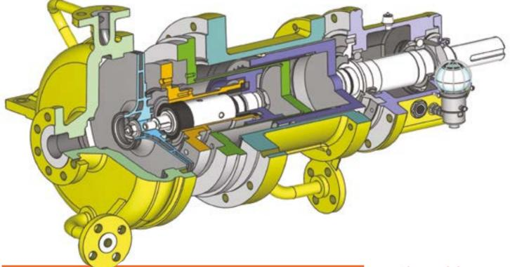
Sundyne HMD have developed comprehensive ranges of horizontal and vertical pumps to fully meet the requirements of 'API 685' without deviation.
