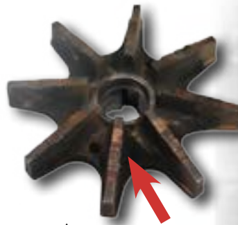
Advanced metal corrosion due to cavitation; under the wrong conditions, cavitation reduces the equipment life time dramatically.
