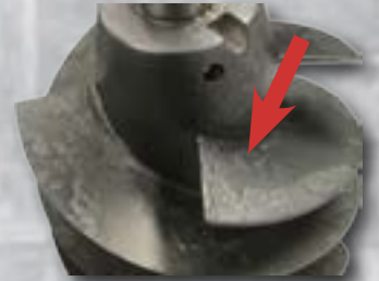
Advanced metal corrosion due to cavitation; under the wrong conditions, cavitation reduces the equipment life time dramatically.
