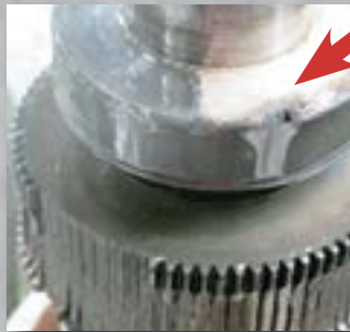
▲ Non-OEM gearbox seals allow process fluid to contaminate lubricant oil.
