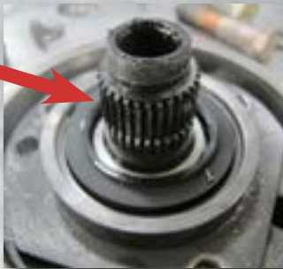
▲ Up thrust failure from non-OEM "re-manufactured" high speed bearing.
